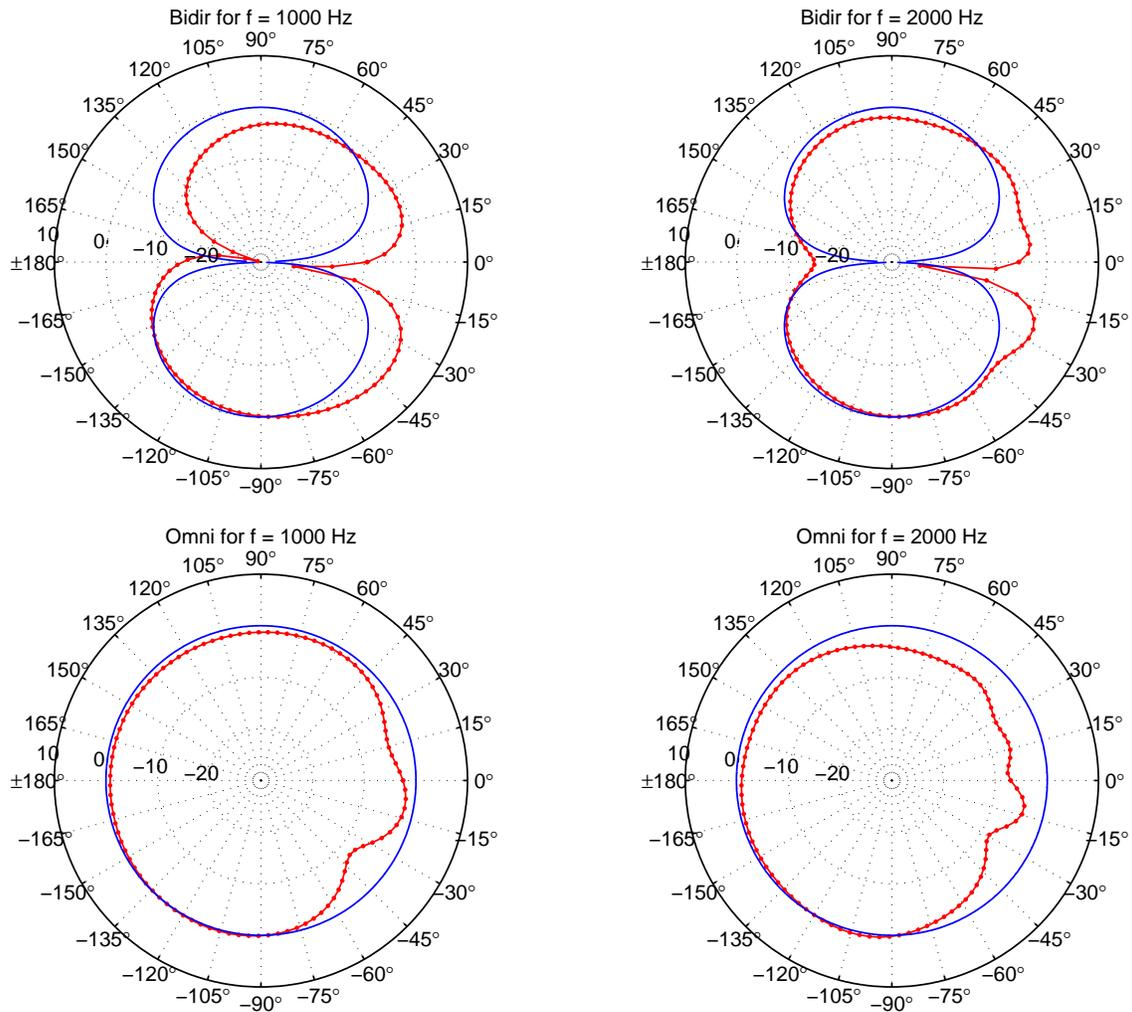
Figure 8: Comparison of the free-field (solid blue line) and the on-the-head (red line with dots) directional characteristics for the HA at a distance of 200 cm. The HA is located on the right ear ( $\pm 180^\circ$ ) and front is towards  $-90^\circ$ .
