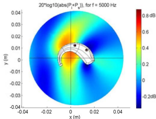
Figure 6: Sound pressure distribution around the HA for  $f = 5000$  Hz. A plane wave is incident from the front (along the x-axis).
