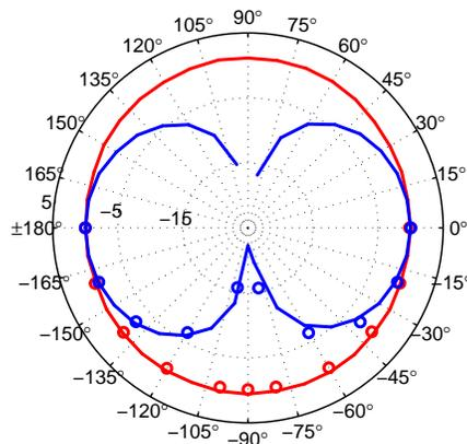
Figure 5: Omni (red) and bidir (blue) response of the HA at  $f = 5000$  Hz. Circle markers represent measurements and the solid line the FE results.
