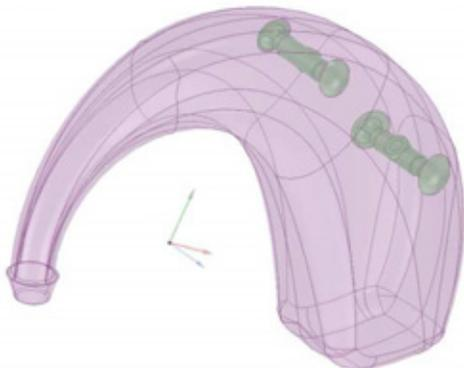
Figure 4: Geometry of the Widex Inteo IN- $m$  hearing aid including the microphone inlets.
