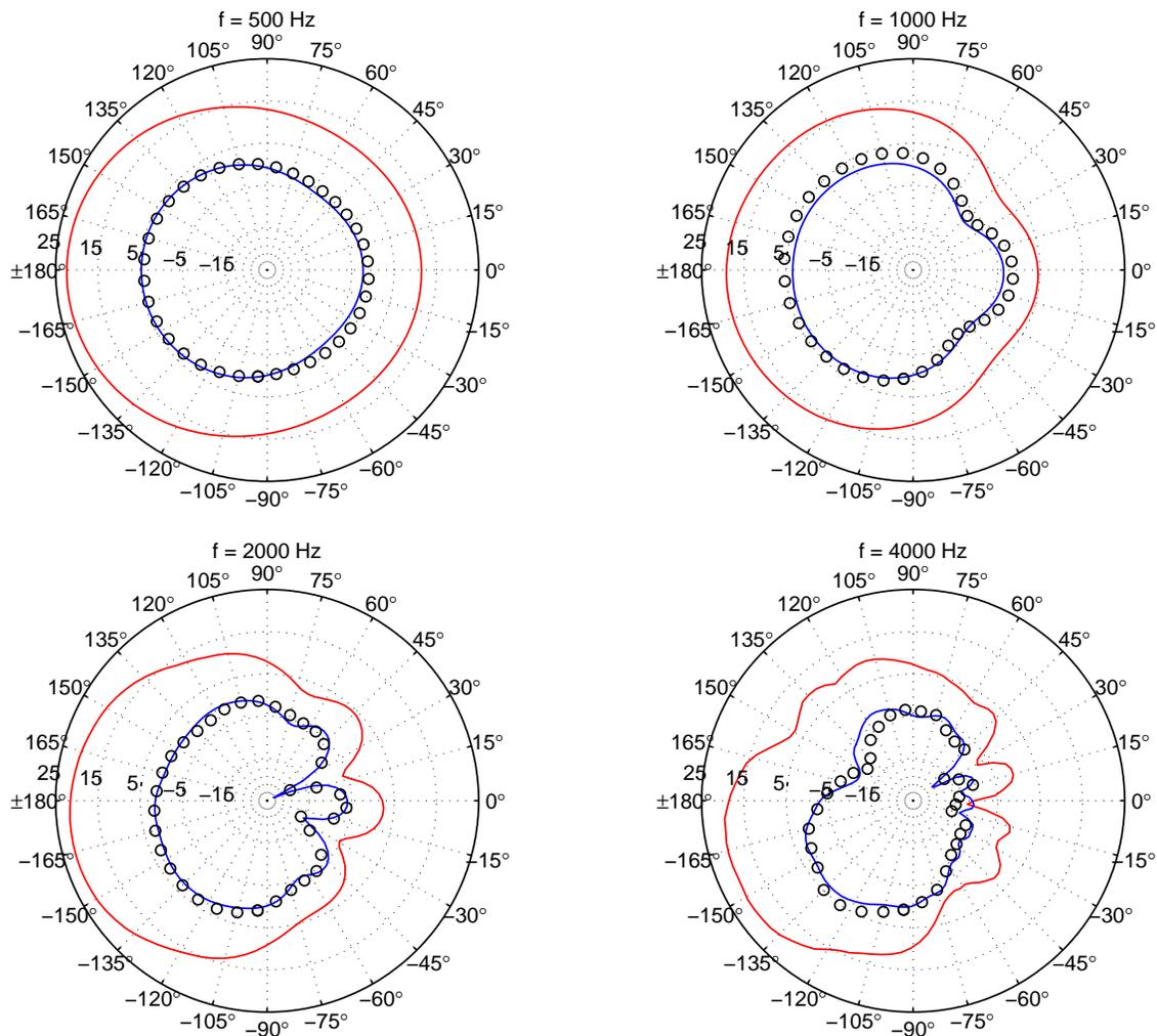
Figure 3: HRTFs of the KEMAR manikin in the horizontal plane with center between the ears. At a distance of 100 cm measurements are given as circles and model results as a blue solid line. The red solid line represents the HRTF at a distance of 20 cm. Front is towards  $-90^\circ$ .
